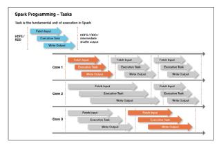
A Spark job using three cores to parallelize output. Up to three tasks run simultaneously, and seven tasks are completed in a fixed period of time. (Source: Lisa Hua, <u>Spark Overview</u>, Slideshare.)
