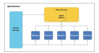
The Spark application is the Driver Process, and the job is split up across executors. (Source: <u>Apache Spark for the</u> <u>Impatient on DZone</u>.)
